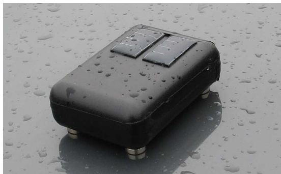
Tracker powered by solar cells
