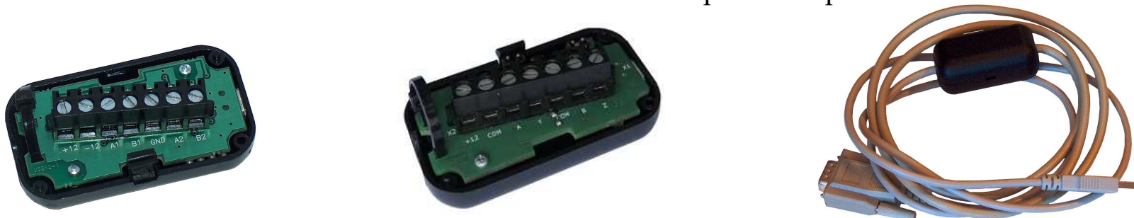
USB - RS485/RS422 converters with power output
