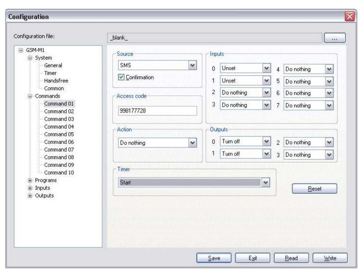
Commands are used for setting/unsetting inputs, turning outputs on or off, starting or stopping timer and handsfree, resetting module. Command's action order is following: reset, timer operation, operation with inputs, operation with outputs, operation with microphone and speaker.
