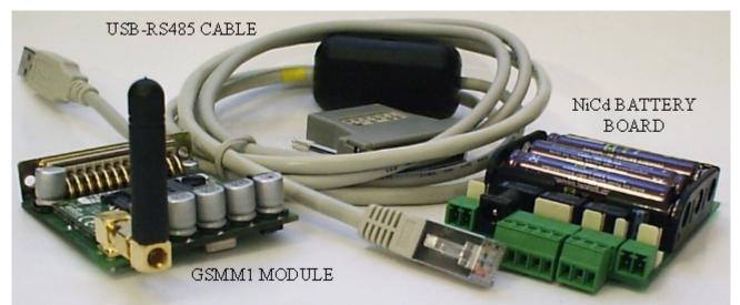
$\mbox{GSMM1/2}$  – 3x or 4x band GSM/GPRS devices, based on ENFORA ENABLER – II G module and ATMEGA128 microcontroller.
