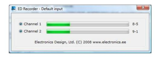
Program is used for recording audio channels into the computer hard drive, audio sources may be one stereo audio or two independent mono channels. Destination format – mp3. Program could recognize outgoing DTMF numbers and incoming CLIP numbers. Attention! Recognition DTMF of parcels probably only at frequency of digitization 8, 16, and 32 kHz.
