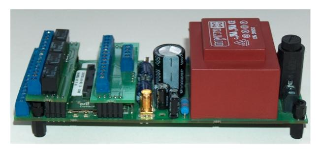
GSMDU is a universal GSM controller which can be used for security, access control, home and industrial automation, data monitoring. For example, automatic phone dialer; communicator with the security panel; remote control for domestic appliances, gate or barrier remote opening; standalone alarm and access control system; etc. It has also built in power supply unit and 12 V battery charger. At the picture GSMDU assembled with plug-in Relay and Auxiliary I/O modules.
